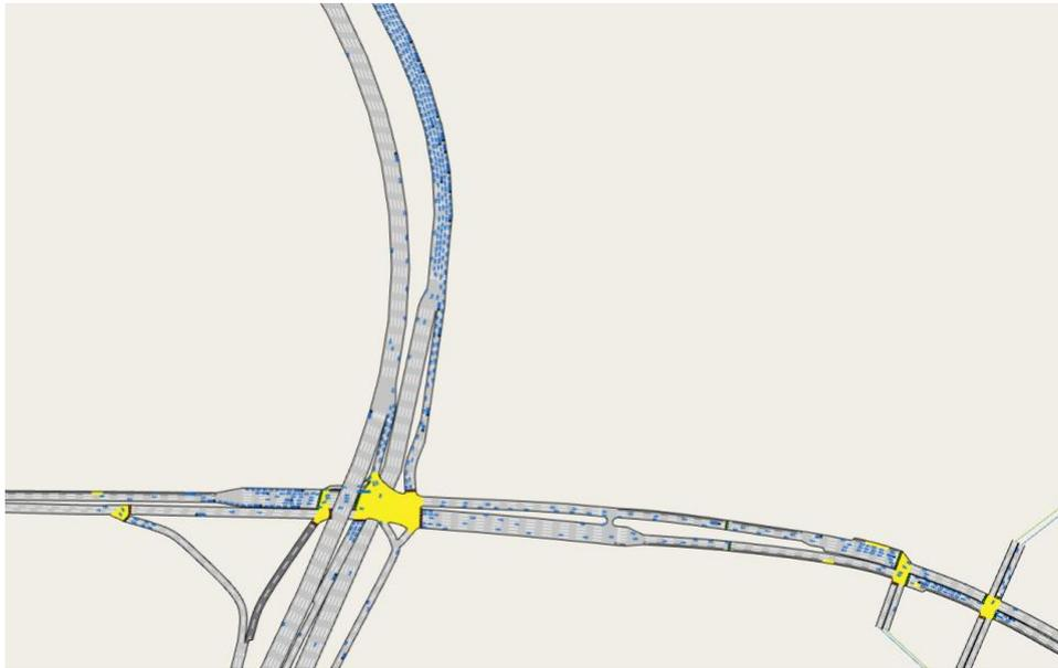
Figure 5.0.2. Simulation: New pile-up on M1 off-ramp after Beaches Link
